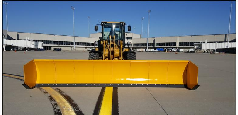
*A 20-foot box plow attached to a wheeled loader.*
