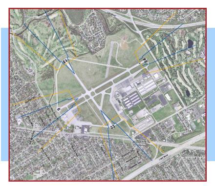
At this time, the FAA is directing the LRAA to focus on the Terminal Instrument Procedure (TERPS) approach surfaces, which are smaller than the previously identified departure surface. This exhibit illustrates a composite of those TERPS approach surfaces, in blue, compared to the TERPS departure surface, in orange.
